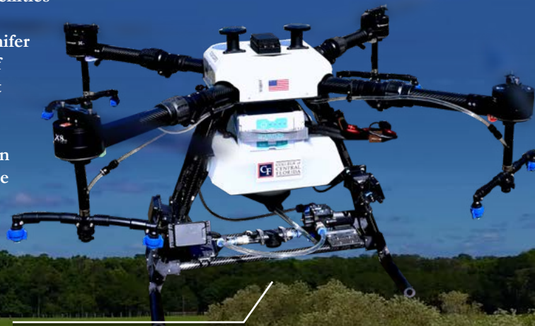
The Hylío Spraying Drone, used for precision crop management, is one of the advanced technologies that give students real-world experience.
